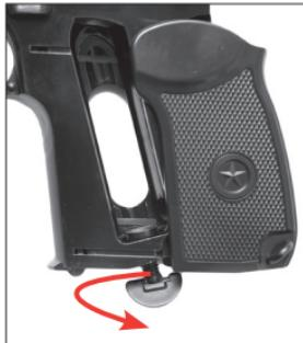
Unscrew cylinder retention screw.
